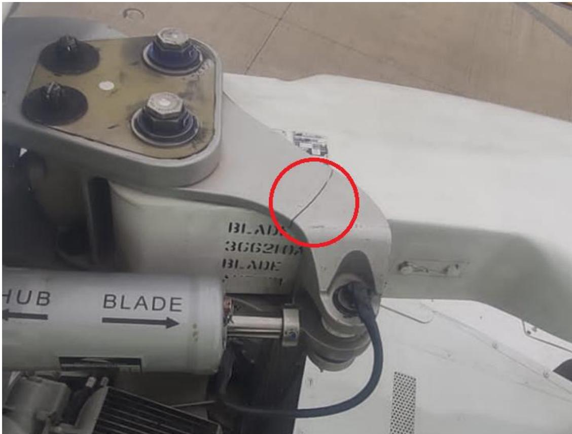
Figura 28: Trinca no Pitch Control Lever
