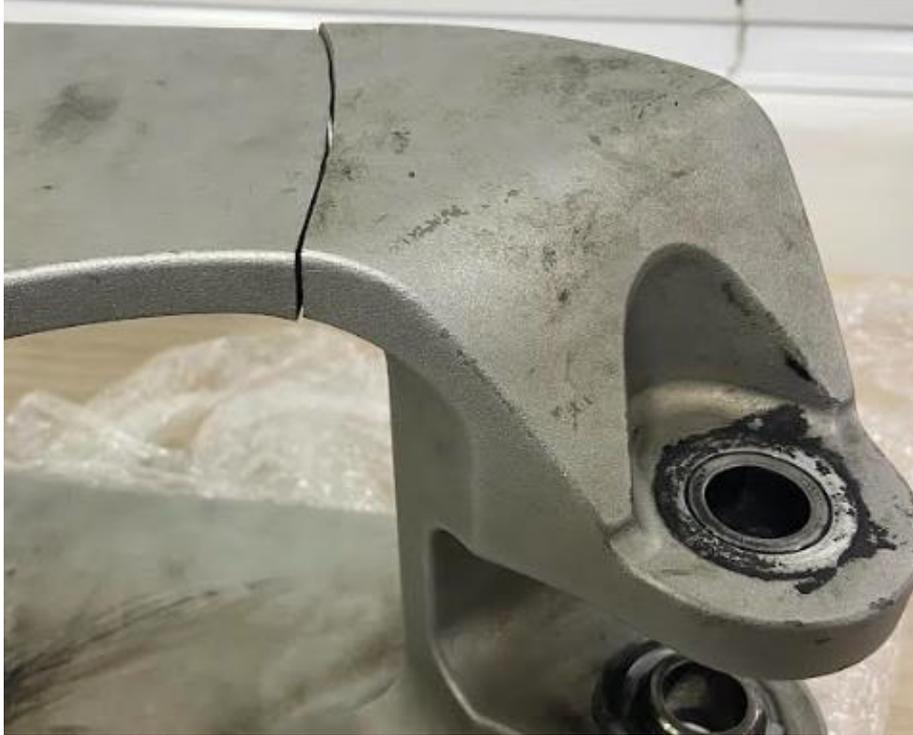
*Figura 29: Fratura no Pitch Control Lever*
